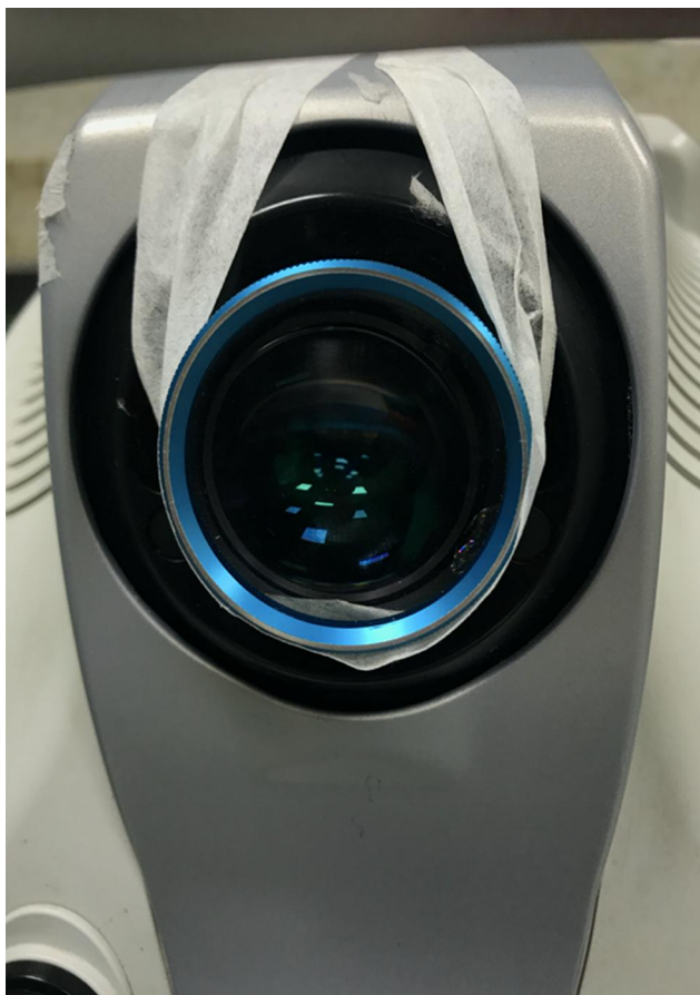
Figure 15 A +20 lens mounted along the aperture of posterior segment OCT using a micropore tape. This will enable anterior segment imaging from the corneal surface to the posterior capsular tip (although not in one frame).
