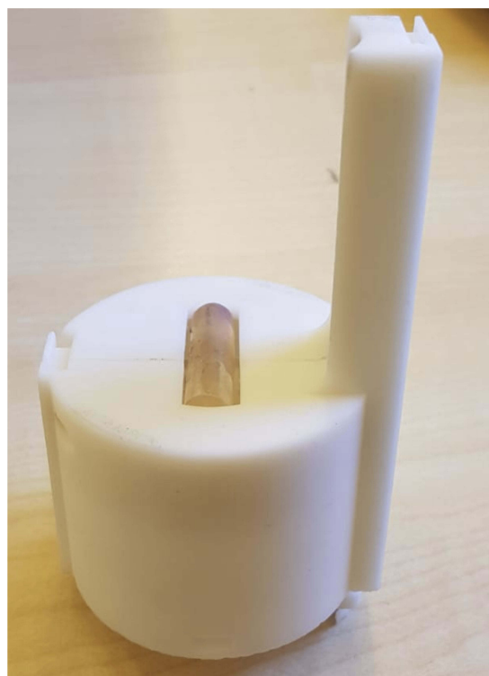
Figure 7 NITINOL switch with a closed shell.
