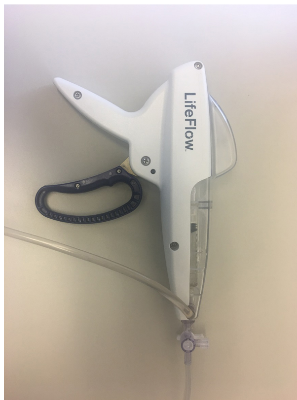
Figure 1 Photograph of the LifeFlow ® Rapid Infuser used in the current study. Note: Although there is proprietary tubing to connect the device to the intravenous cannula, we chose to use a 33 inch extension tubing with a three-way Hi-Flo stopcock to connect the device to the intravenous cannula to keep the tubing standardized across the two delivery systems.
