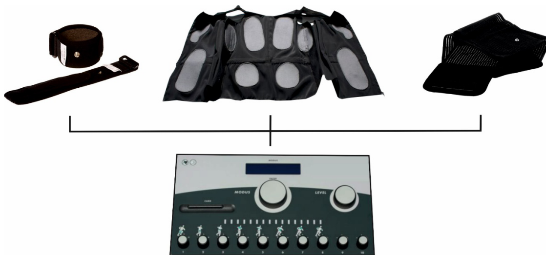
Figure 2 WB-EMS equipment with operator device and electrodes (vest, arm-, leg-, gluteal-cuffs). Abbreviation: WB-EMS, whole-body electromyostimulation.
