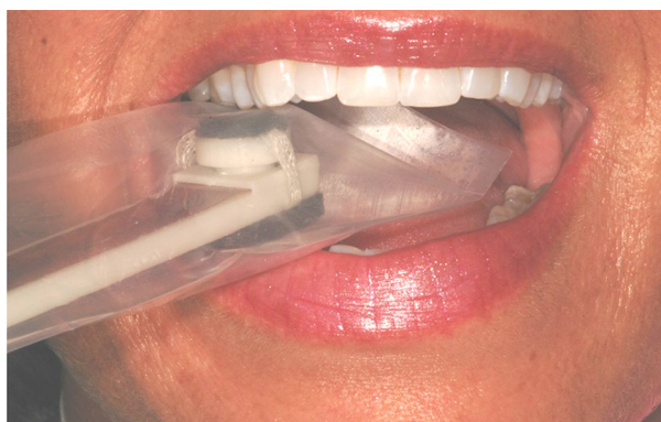
Figure 9 The pressure sensor is placed in the patient's mouth in the site where the loading will occur and the patient is instructed to bite with maximum force.
