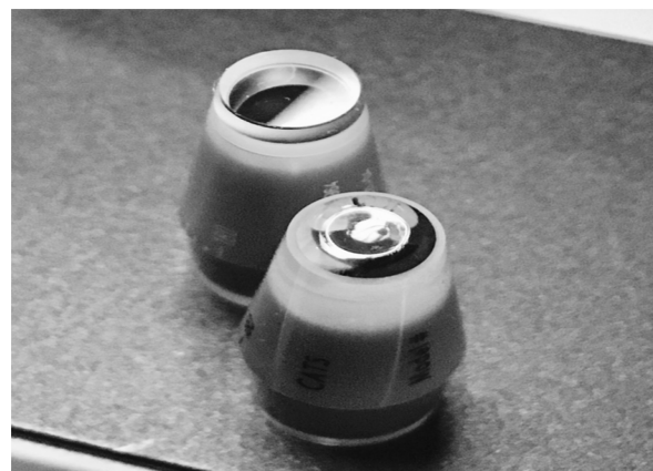
Figure 2 Photograph of the CATS tonometer prism applanating surface. Abbreviation: CATS, correcting applanation tonometry surface.
