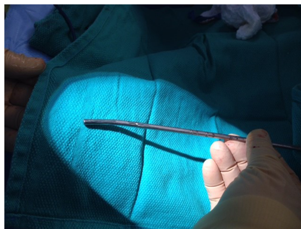
Figure 4 This image shows in situ wear on the rod from the Shilla screw.
