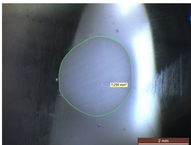
Figure 7 Measurement of a cut state-of-the-art Y-TZP FDP core under light microscope.
