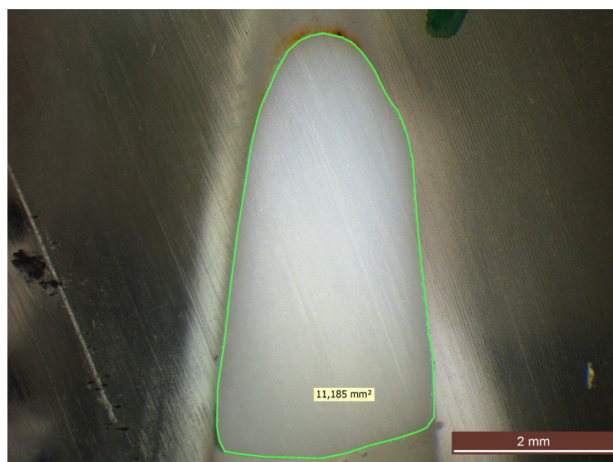
Figure 6 Measurement of a cut split-file Y-TZP FDP core under light microscope. Notes: The figure shows the cross-section area of the connector between the central incisor and pontic. Abbreviations: FDP, fixed dental prosthesis; Y-TZP, yttria-stabilized tetragonal zirconia polycrystal.
