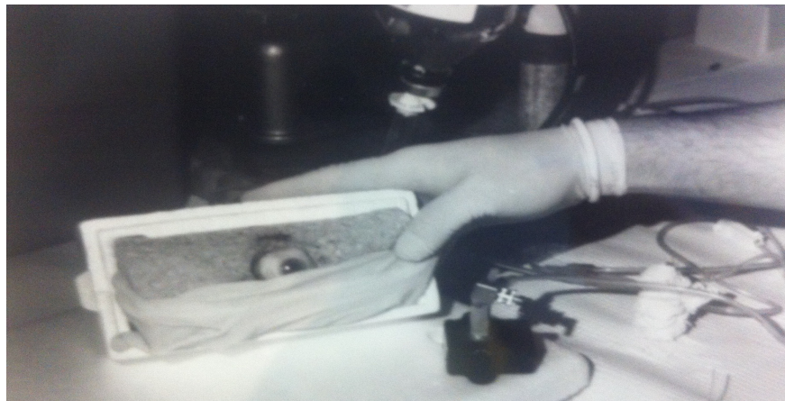
Figure 4 A fresh human cadaver eye was mounted within a mock orbit that consisted of a Styrofoam box filled with a moist sponge.
