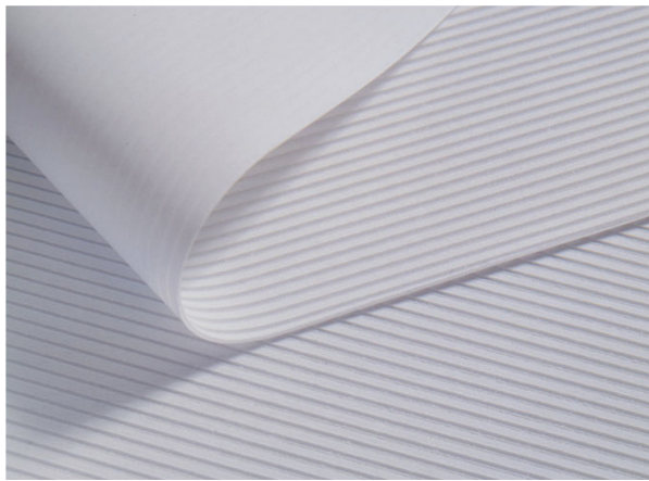
Figure 4 Photograph showing the textured and smooth dual surface of the MVP® sheet magnified under a microscope. Note: Each strip is 0.8 mm in length.
