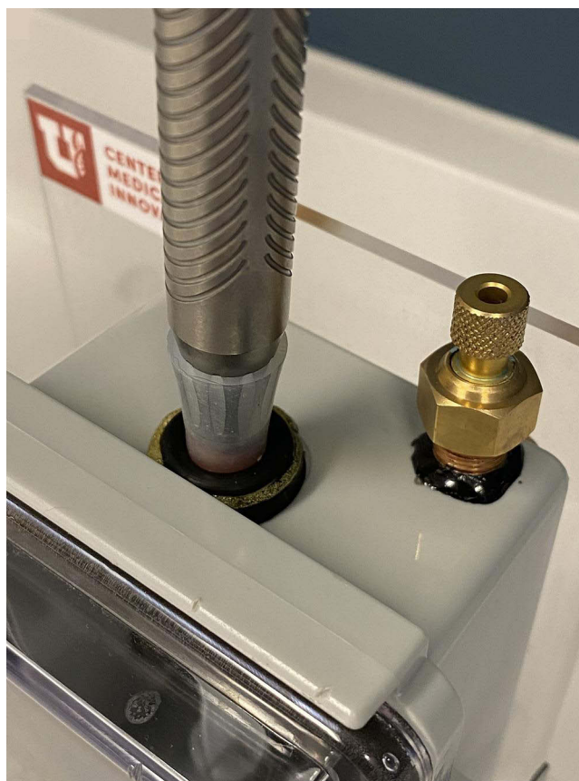
Figure 2 Close-up photograph of the pressure chamber detailing the phacoemulsification handpiece insertion point, which seals to create a watertight barrier around the handpiece. The brass fitting serves as a bleed valve, used to evacuate air from the chamber and normalize intra-chamber pressure between trials.
