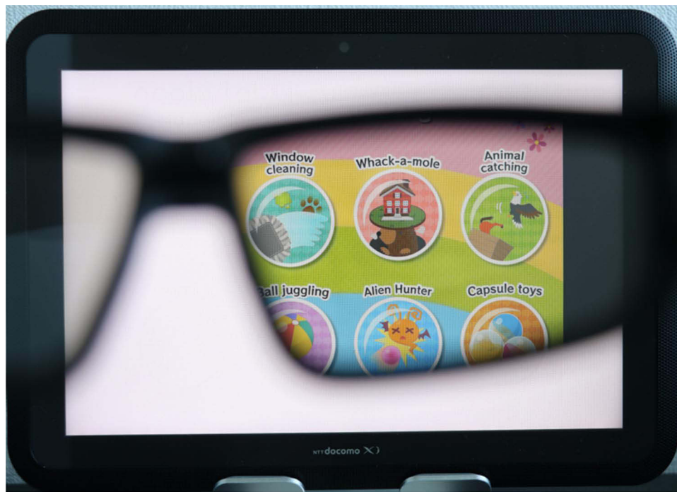
Figure 1 Image of the Occlu-tab device. The Occlu-tab enables visual stimulation of one eye when viewed through polarized glasses. The designated training eye can perceive the displayed images through the polarized glasses, whereas the fellow eye cannot. The images displayed on the liquid crystal screen are not visible to the naked eye.
