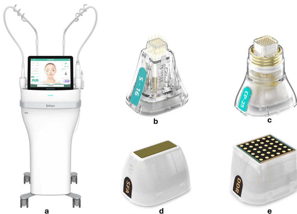
Figure 1 (a) POTENZA™ RFMN System, (b) Semi-insulated invasive tip S-16, (c) Pumping Tip CP-25, (d) noninvasive superficial ablation SFA Tip, and (e) deep dermal rejuvenation DDR Tip.
