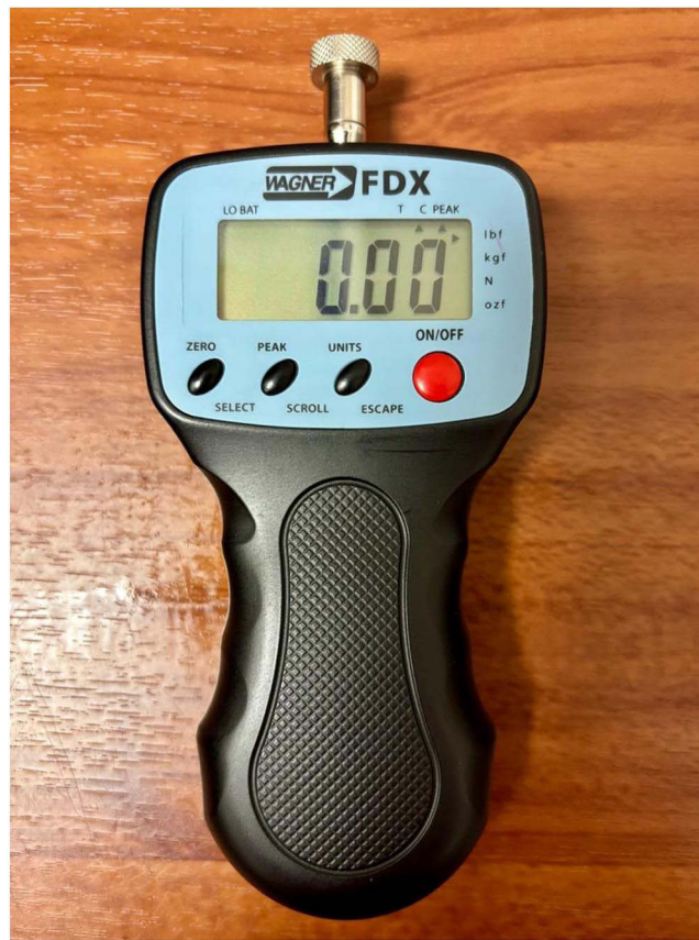
Figure 1 Electronic pressure algometer used for experimental pain induction in pressure pain threshold and conditioned pain modulation testing.
