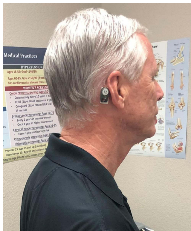
Figure 1 Phybrata sensor attached to the mastoid using an adhesive patch.
