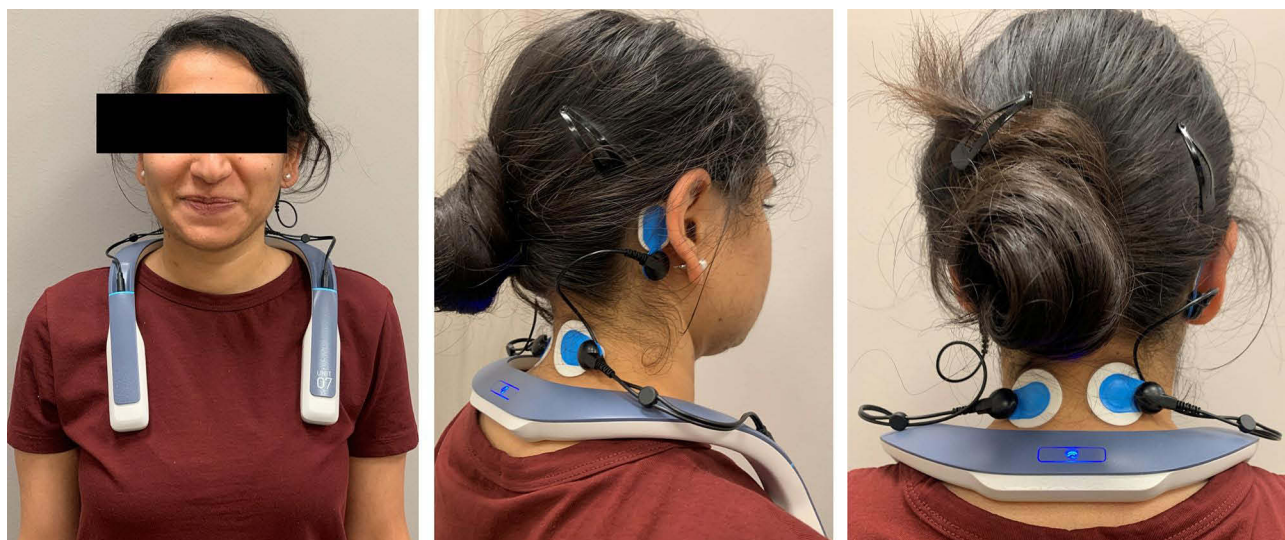
Figure 2 NEURVESTA device attached using disposable electrodes.
