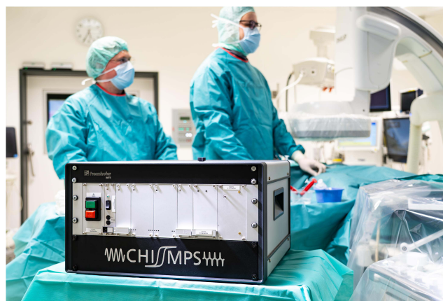
Figure 1 The used magnetic particle spectrometer “CHIMPS” (foreground) at the bedside in a clinical setting for endovascular interventions (background). The image depicts the anticipated application for continuous monitoring of patient coagulation status.
