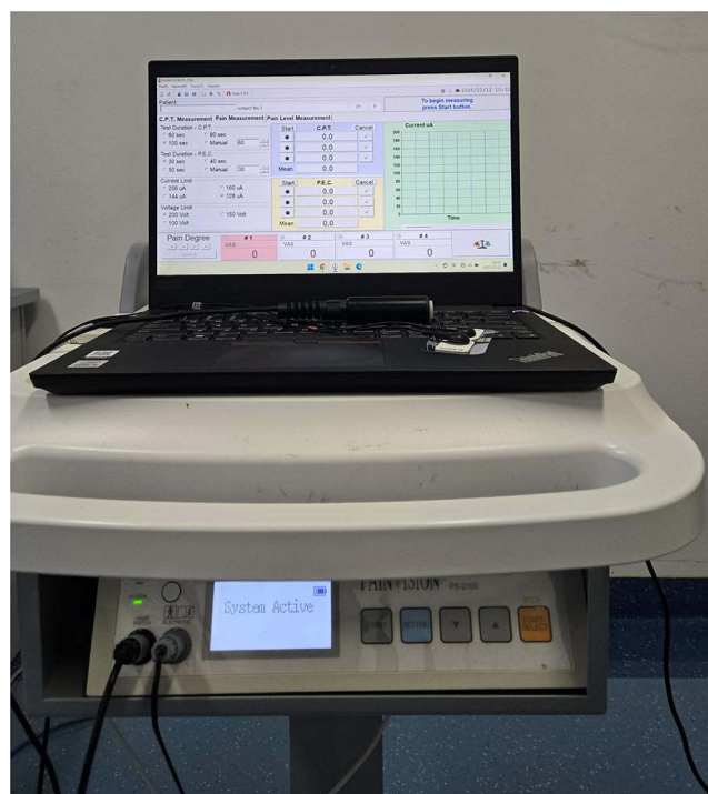
Figure 2 PainVision® PS-2100 apparatus used for measuring electrical detection threshold and electrical pain threshold.
