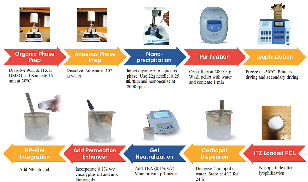
Figure 1 Schematic Diagram of the Nanoprecipitation Method for ITZ-PCL Nanoparticle Preparation.
