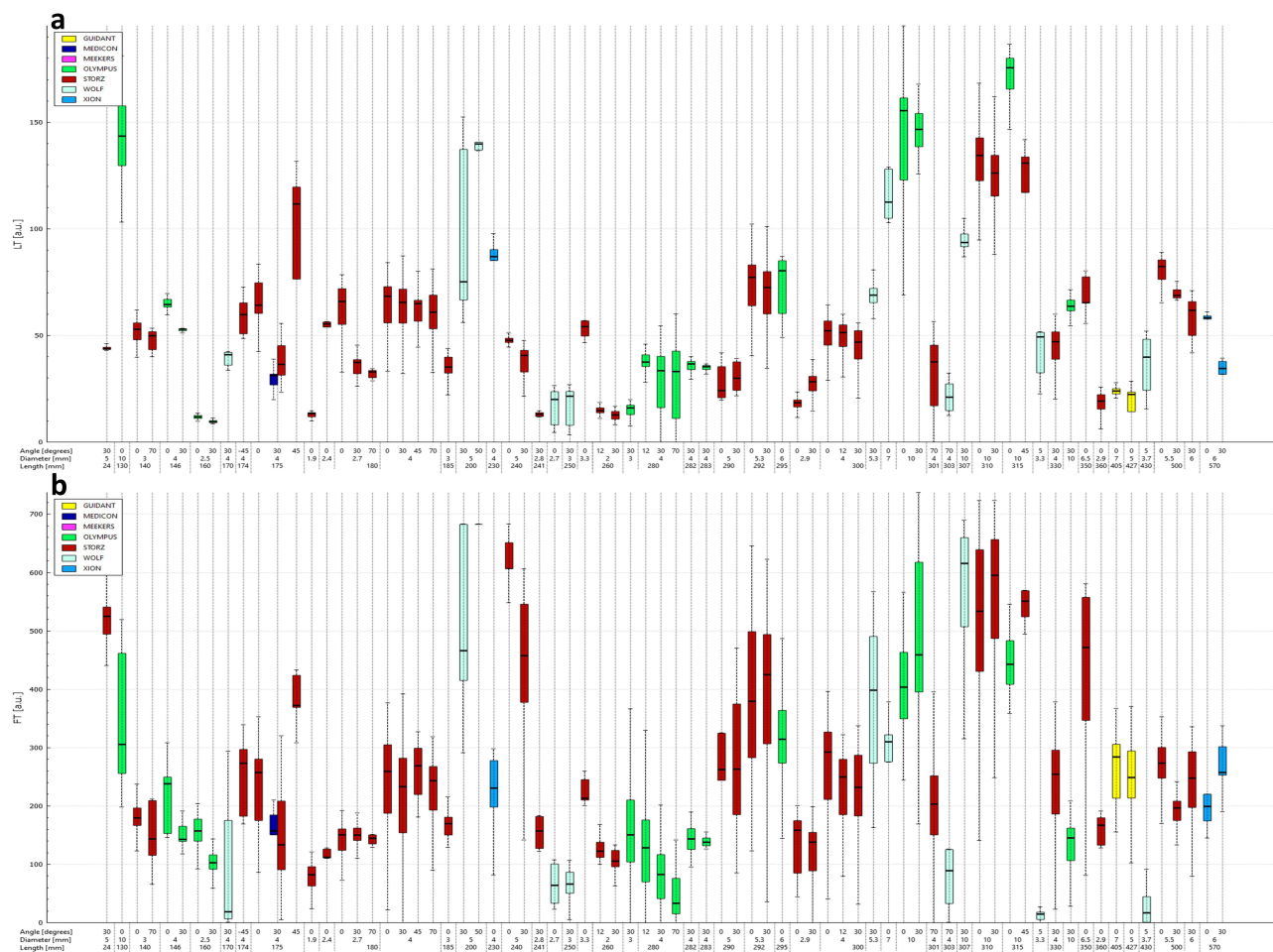
Figure 8 Start LT and FT values for the seven major brands in all hospitals are arranged by length, diameter, and view angle. Clearly, thicker endoscopes have higher LT and FT values. There are almost no endoscopes (with sufficient data) from different brands with the same specifications, which makes comparison difficult. A comparison can be made for endoscopes that are 175 mm long, 4 mm wide, and have a 30-degree angle. In this case, Storz endoscopes seem to have a larger start LT value than the Medicon alternative, but this might be explained by an (unknown) larger field of view.
