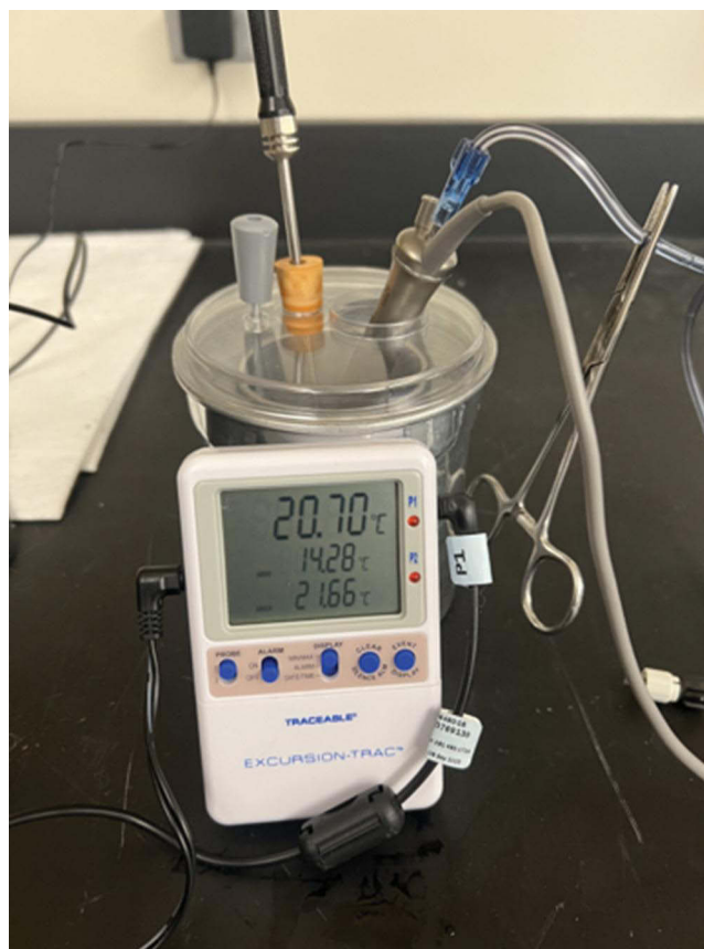
Figure 1 Experimental setup showing calorimeter, temperature probe, handpiece with hemostat, and stirring rod.
