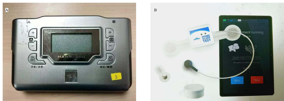
Figure 2 Han's acupoint nerve stimulator. (A) HANS200A (the device for TEAS application); (B) The self-adhesive gel electrodes.
