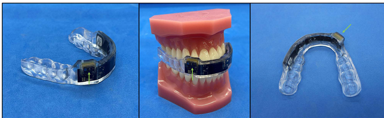
Figure 1 The buccal mucosal oximeter device. The photoplethysmography (PPG) unit is indicated by the green arrows.
