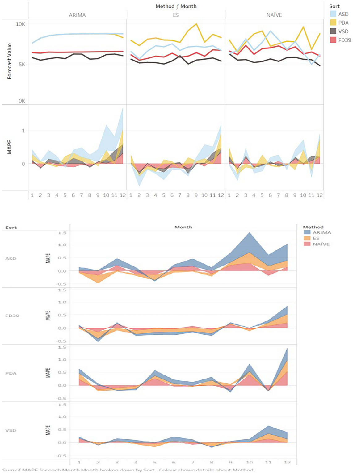
Figure 3 Visual comparison of three forecast methods MAPE. The upper part of the figure shows the forecast results and MAPE trend charts of different diseases using ARIMA, ES, and Naive forecast methods. The lower part shows the MAPE performance of the three forecast methods mentioned above in different diseases, which determines the degree of deviation between the forecast and actual values based on the size of the area.
