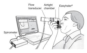
Figure I The Easyhaler inhaler connected in series to a pneumotachograph.
