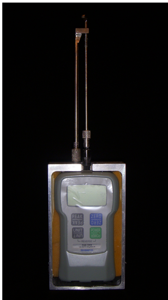
Figure 1 The Digital Force Gauge and its components.
