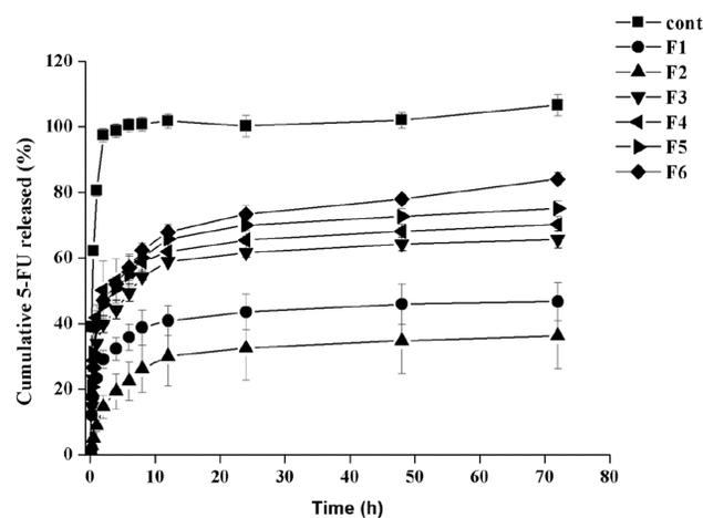
**Figure 4** Release profiles of 5-FU from loaded nanoparticles in phosphate buffer pH 7.4 through dialysis bags with cut-off 12,000 Dalton using 5-FU aqueous solution as a control (mean  $\pm$  SD, n = 3).
