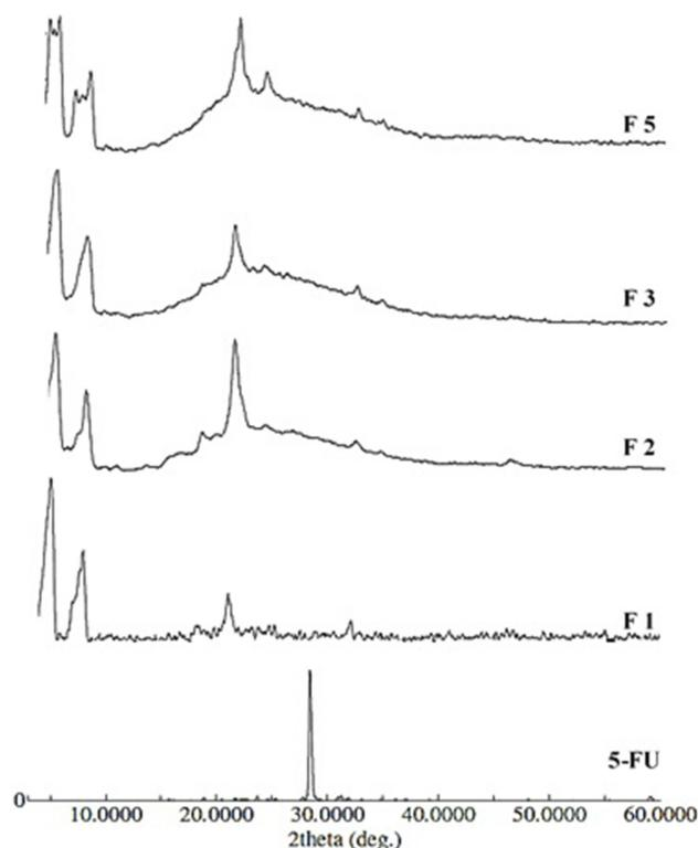
**Figure 2** XRD diffractograms of pure 5-FU and 5-FU-loaded nanoparticles.
