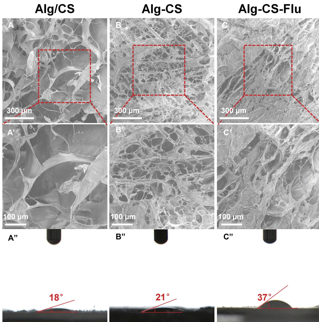
**Figure 2** Surface SEM images and WCAs (images of drops captured at 0.5 s) of scaffolds: (A), (A'), and (A'') Alg/CS scaffold; (B), (B'), and (B'') Alg-CS scaffold; (C), (C'), and (C'') Alg-CS-Flu scaffold.
