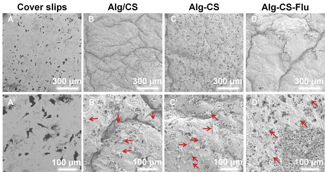
**Figure 8** SEM micrographs of L929 cells grown onto (A and A') coverslips; (B and B') Alg/CS scaffold; (C and C') Alg-CS scaffold; (D and D') Alg-CS-Flu scaffold after 5-d culture. (A–D) magnified 200 times; (A'–D') magnified 500 times. The red arrows represent L929 cells.
