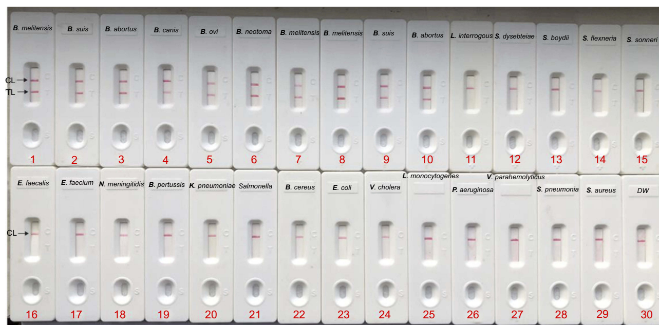
Figure 6 Specificity of Brucella -LAMP-LFB assay using different bacterial strains. The Brucella -LAMP-LFB was tested using different genomic DNAs. Biosensor 1, B. melitensis (GZ-CDC-M5); biosensor 2, B. suis (GZ-CDC-S2); biosensor 3, B. abortus (GZ-CDC-A19); biosensor 4, B. canis (isolated strain); biosensor 5, B. ovi (isolated strain); biosensor 6, B. neotoma (isolated strain); biosensor 7–8, B. melitensis (isolated strains); biosensor 9, B. suis (isolated strain); biosensor 10, B. abortus (isolated strain); Biosensor 11–29, Leptospira interrogans ; Shigella dysenteriae ; Shigella boydii ; Shigella flexneria ; Shigella sonnei ; Enterococcus faecalis ; Enterococcus faecium ; Neisseria meningitidis ; Bordetella pertussis ; Klebsiella pneumoniae ; Salmonella ; Bacillus cereus ; Enterotoxigenic E. coli ; Vibrio cholera ; Listeria monocytogenes ; Pseudomonas aeruginosa ; Vibrio parahaemolyticus ; Streptococcus pneumoniae ; Staphylococcus aureus ; Biosensor 30, negative control (DW).
