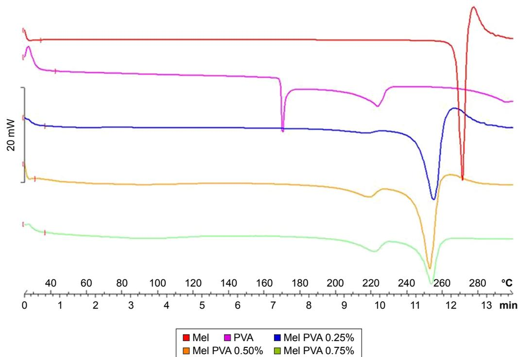
**Figure 7** DSC curves of raw Mel and PVA and dried dispersions with different PVA concentrations.
