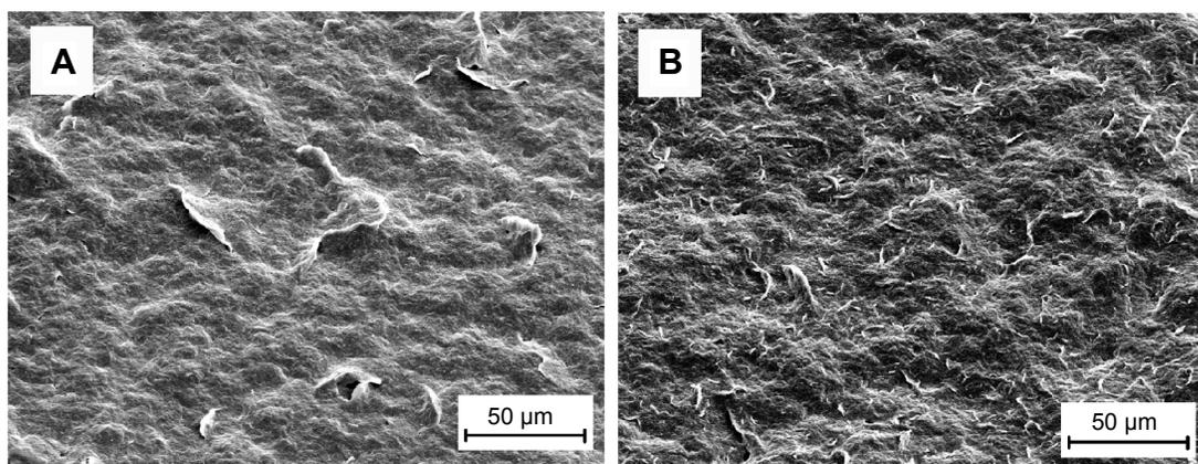
**Figure 4** Scanning electron micrographs of E7-PLLA<sub>sc</sub> (A) and E7-APLLA<sub>sc</sub> (B) aggregates.
