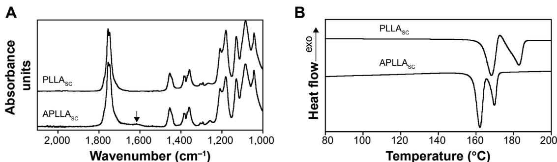
**Figure 2** Attenuated total reflection Fourier transform infrared spectra of PLLA<sub>sc</sub> and APLLA<sub>sc</sub> (A). Differential scanning calorimetry thermograms of PLLA<sub>sc</sub> and APLLA<sub>sc</sub> recorded at 10°C per minute (B).
