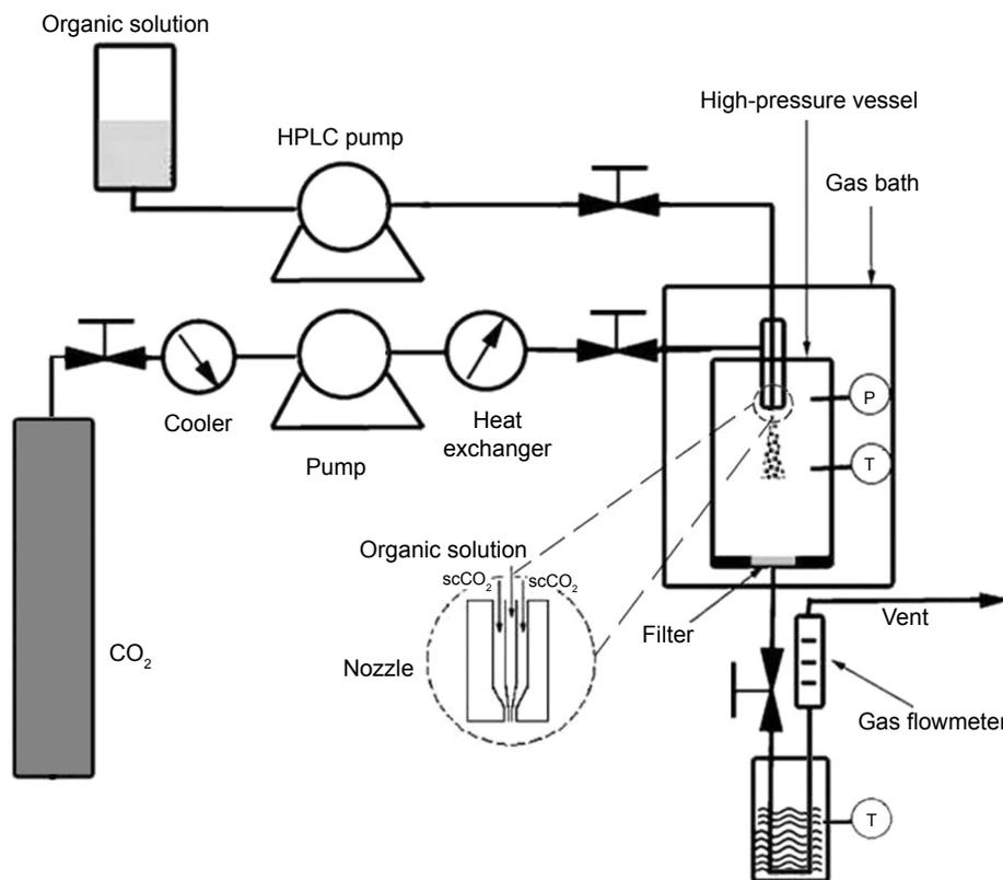
**Figure 1** Schematic diagram of the SEDS process.
