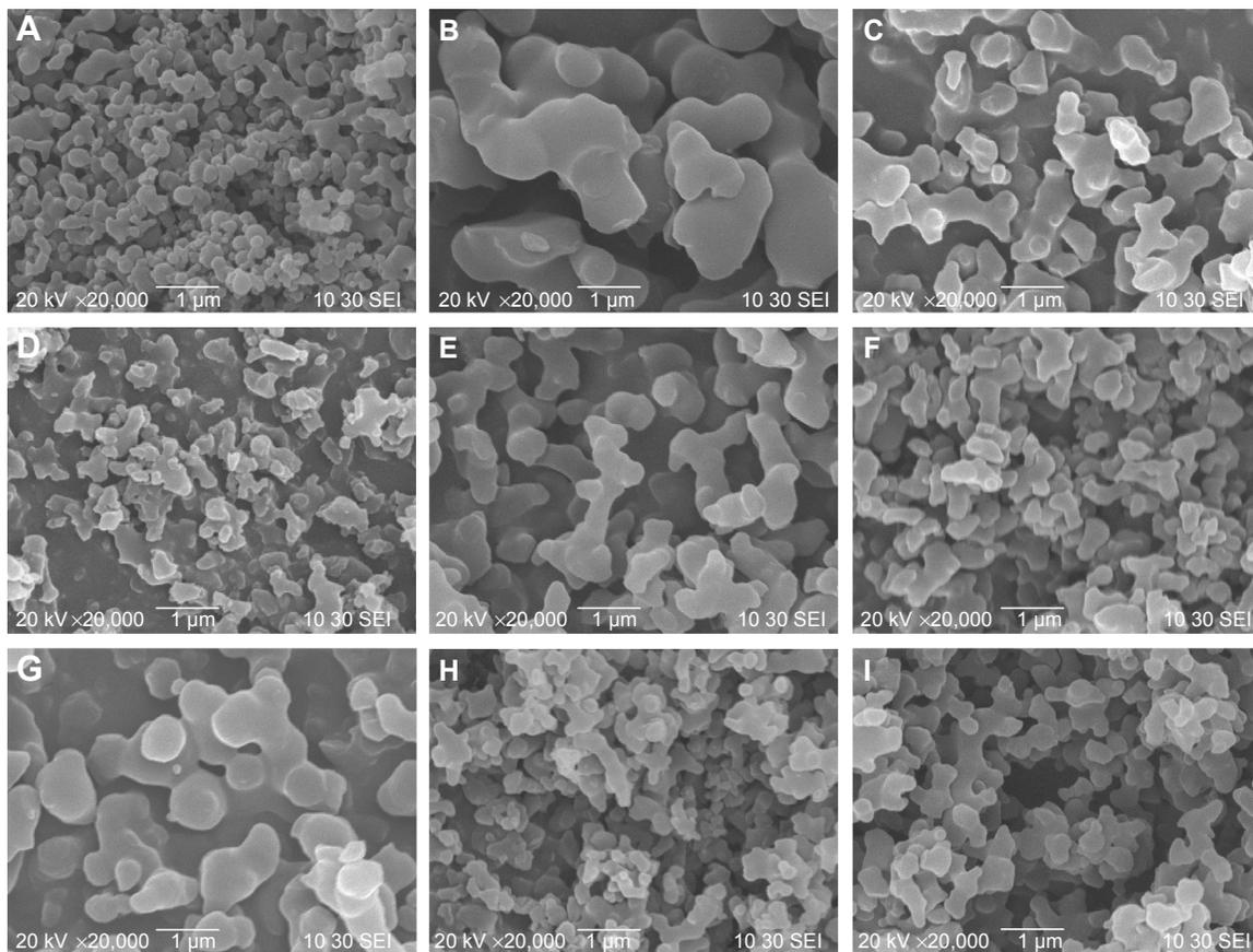
**Figure 3** SEM micrographs of curcumin nanoparticles prepared by the SEDS process under different conditions (A) 0.5%-35°C-0.5 mL/min-20 Mpa; (B) 0.5%-45°C-1 mL/min-10 Mpa; (C) 0.5%-45°C-0.5 mL/min-10 Mpa; (D) 5%-45°C-0.5 mL/min-20 Mpa; (E) 0.5%-35°C-1 mL/min-10 Mpa; (F) 1%-45°C-0.5 mL/min-20 Mpa; (G) 1%-45°C-1 mL/min-20 Mpa; (H) 1%-35°C-1 mL/min-20 Mpa; (I) 0.5%-35°C-1 mL/min-20 Mpa.
