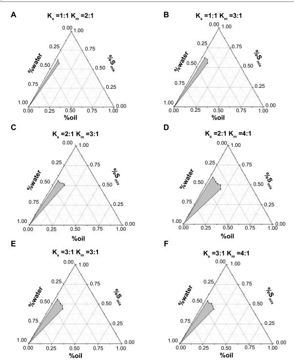
Figure I Pseudoternary phase diagram of the different S<sub>mix</sub> systems containing the oil phase (Labrafil®), surfactants (Labrasol® and Cremophor® RH40), cosurfactant (Transcutol® HP), and aqueous phase (distilled water).
