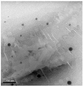
Figure 5 Transmission electron microscopy of the rotigotine-loaded microemulsion.
