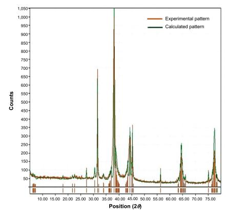
Figure 6 X-ray diffraction spectrum of green-synthesized silver nanoparticles.
