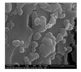
**Figure 3** Scanning electron microscopic image of green silver nanoparticles synthesized by reduction of aqueous AgNO<sub>3</sub> ions using aqueous extract of *Gymnema sylvestre*. **Abbreviations:** HV, high voltage; WD, working distance; mag, magnification; ETD, Everhart–Thornley detector.
