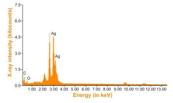
Figure 4 Energy-dispersive X-ray spectrum of green silver nanoparticles.
