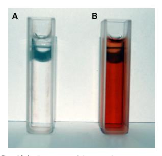
Figure I Surface plasmon resonance of silver nanoparticles. Notes: (A) silver nitrate solution; (B) green-synthesized silver nanoparticles in ruby red color after 30 minutes.
