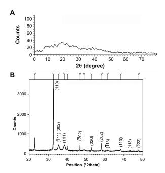
**Figure 2** XRD pattern of synthesized CuO nanoparticles. XRD pattern of (**A**) GK and (**B**) CuO nanoparticles, indicating the amorphous nature of GK and the crystalline nature with different planes of synthesized CuO nanoparticles. **Abbreviations:** XRD, X-ray diffraction; GK, gum karaya; CuO, copper oxide.
