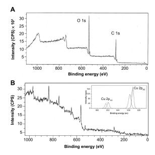
Figure 5 XPS survey scanning spectra of the ( $\bf A$ ) GK ( $\bf B$ ) GK-CuO nanoparticles formation.
