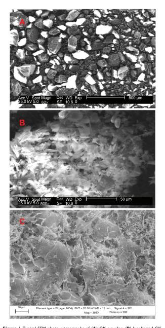
Figure 1 Typical SEM photo micrographs of (A) GK powder, (B) lyophilized GK, and (C) synthesized CuO nanoparticles.
