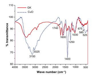
**Figure 3** FTIR analysis of GK and CuO nanoparticles indicating the involvement of various functional groups in the formation of metal oxide nanoparticles. **Abbreviations:** FTIR, Fourier transform infrared spectroscopy; GK, gum karaya; CuO, copper oxide.
