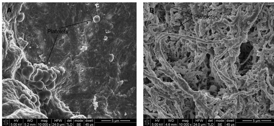
**Figure 7** SEM images (5000 $\times$ ) of platelets adhering to the surface of unmodified (A) and heparin/DHI-modified bovine jugular vein scaffolds (B).
