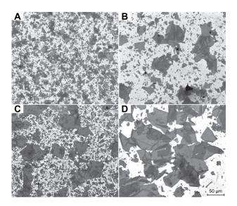
**Figure I** Field emission scanning electron microscopy micrographs of graphene oxide prepared in (A) KS-80, (B) KS-40, and (C) KS-20 after 3 days of oxidation and (D) nonsonicated KS-20. All the micrographs were taken at the same magnification.
