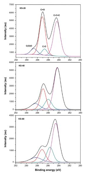
**Figure 4** X-ray photoelectron spectrometry analysis of graphene oxide with different degrees of oxidation illustrating the deconvoluted X-ray photoelectron spectra in the C1s peak region for the KS-20, KS-40, and KS-80 samples.
