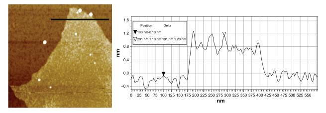
Figure 2 Atomic force microscopy measurement of graphene oxide (scan area: 1 µm × 1 µm). Tapping mode atomic force microscopy image of single-layer graphene oxide (KS-20) with corresponding height cross-sectional profile with an average thickness of 1.2 nm. The sample was spin-coated on a freshly cleaved mica substrate.
