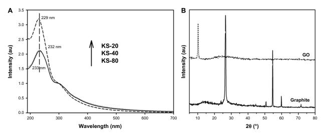
Figure 3 (A) Ultraviolet-visible absorbance spectra of graphene oxide after 3 days of oxidation time, and (B) X-ray diffraction patterns of graphite flakes and graphene oxide.
