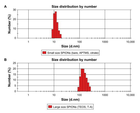
Figure SI Size distributions of relatively small SPIONs (ie, bare and APTMS- or citrate-coated) (A) and large SPIONs (ie, TEOS- or T-A-coated) (B) in aqueous solution. Note: The Zetasizer histograms shown in this figure are representative of five independent experiments with almost similar results. Abbreviations: APTMS, (3-aminopropyl)trimethoxysilane; DMSO, dimethyl sulfoxide; SPION, superparamagnetic iron oxide nanoparticles; T-A, TEOS-APTMS; TEOS, tetraethyl orthosilicate.
