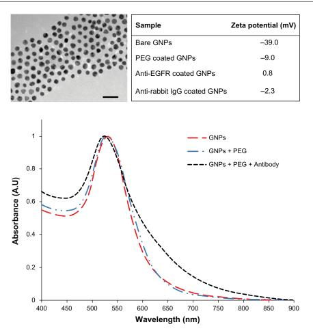
Figure I Characterization of gold nanoparticles (GNPs). Upper left: transmission electron microscopy image of 30 nm GNPs (scale bar 100 nm). Upper right: zeta potential measurements at the various stages of GNP coatings. Bottom: ultraviolet-visible spectroscopy of the bare GNPs, polyethylene glycol (PEG)ylated GNPs, and anti-epidermal growth factor receptor (EGFR)-coated GNPs. **Abbreviations:** A.U, abitrary unit; IgG, immunoglobulin G.
