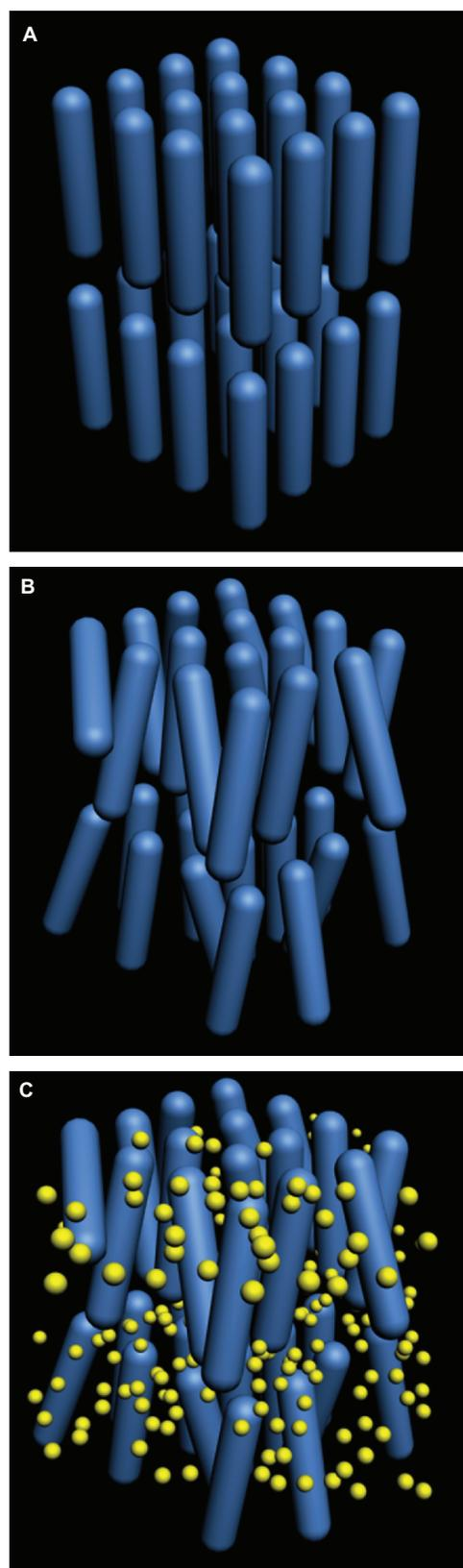
**Figure 2** (A) The rod-like molecules of mesogenic unit of ALCRM and (B) the arrangement of the rod-like molecules during polymerization; (C) na-HA filler (yellow sphere) reinforce the rod-like structure.
